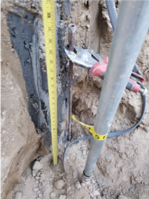
Photo 2: Metal probe fully inserted into the annulus. Note measurement to vice gripe.
