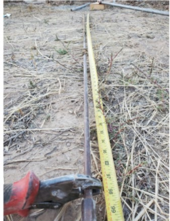
Photo 3: Metal probe extracted and measured to vice gripe.
